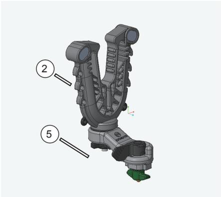
// Loosen Lock Knob (5) and rotate FlexGrip (2) to the desired angle, Tighten Lock Knob (5)
